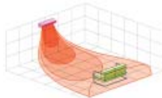
Floor level heating When required, the power diffuser automatically opens, concentrating airflow down to the floor level.
